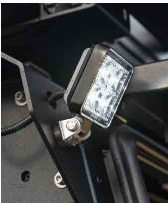
External Camp / Work Lighting
